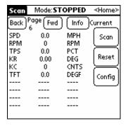
The final sample page is an example of how you might diagnose engine knock (pinging). You can log these parameters and determine under what conditions – speed, rpm, throttle position – the knock retard (KR) is occurring.
